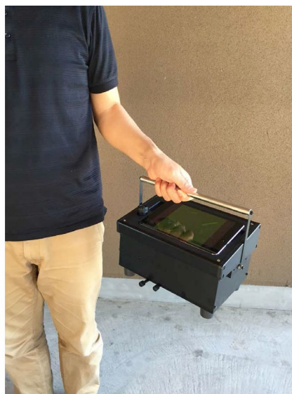
Figure 4. Development of portable fluorescence microscope for on-site detection of asbestos. The compact and portable fluorescence microscope was designed by a Hiroshima University spin-off venture Siliconbio Inc. (Higashi-Hiroshima, Japan) in collaboration with Opto Science Inc. (Tokyo, Japan). The microscope contains a blue LED excitation light source (470 nm, 200 mW) with a constant current output driver, a 470-nm narrow band excitation filter (470QM40, Omega), a dichroic mirror with cutoff at 505 nm (505DRLP, Omega), and a 20× objective lens ( NA = 0.40 , f = 3.32 mm) with a 510 nm long-pass fluorescence filter (510QMLP, Omega). The device does not have a dedicated CCD unit, relying instead on an iPad camera module. A demonstration video is available at the following website: http://siliconbio.co.jp .
